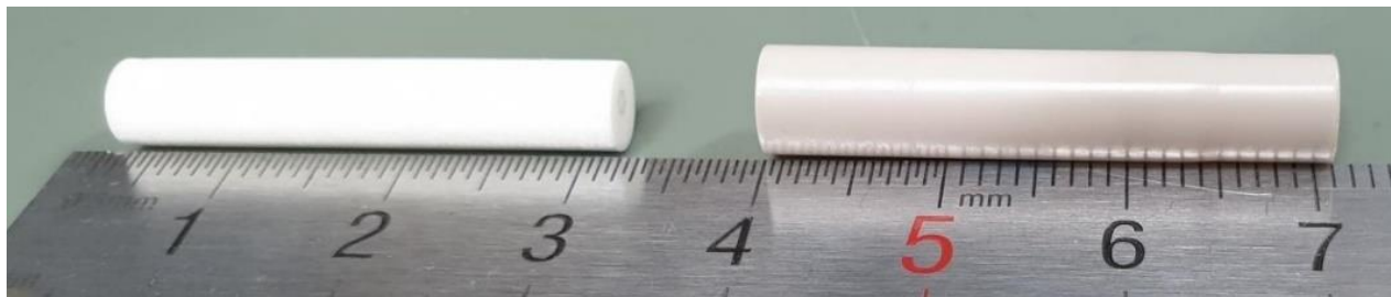
Figure 3. Commercially of the shelf available regenerator material and displacer tube prior to assembly
