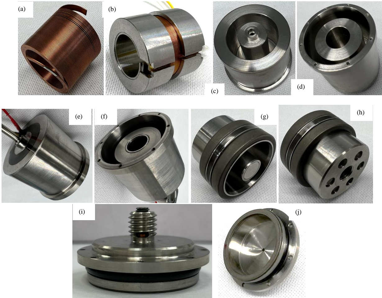
Figure 22. Compressor: components and subassemblies
