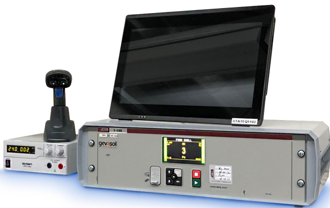
A typical workstation, including a leak detector, Mini PCs, and scanner.
